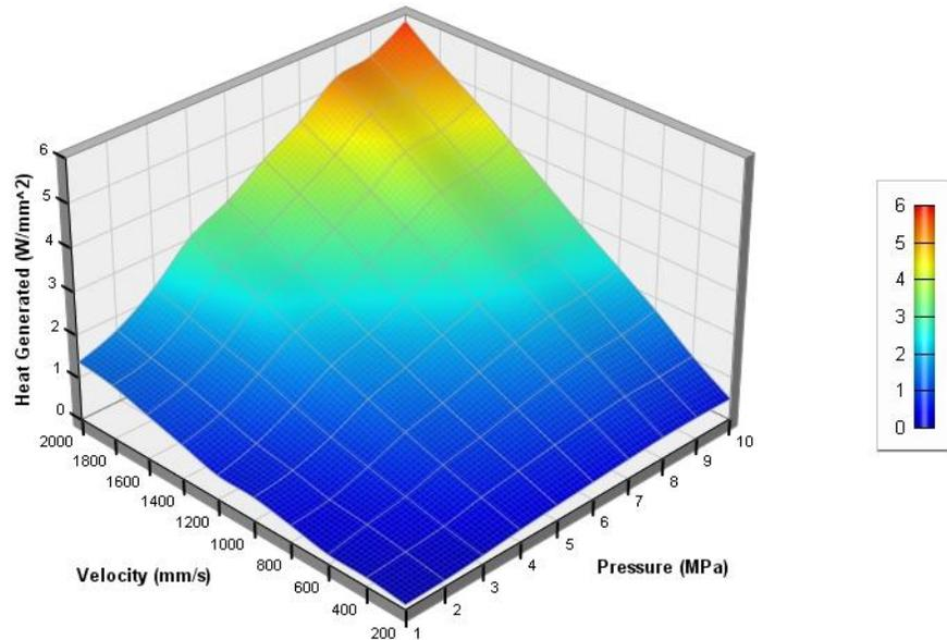
The published P-V limit for this material is 10,000 psi\*ft/min. This corresponds to heat generation less than 0.1W/mm<sup>2</sup> at the frictions measured.
