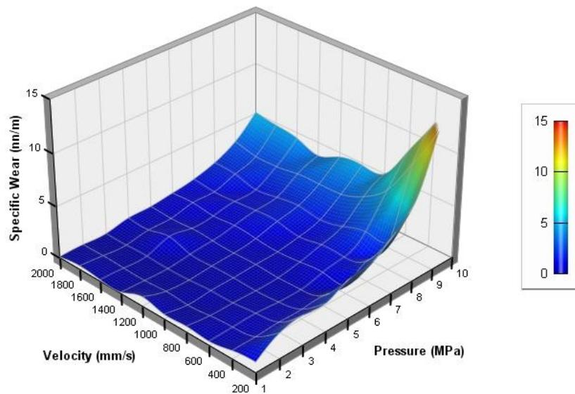
Wear can be considered acceptable for some P-V combinations up to 20 W/mm<sup>2</sup> (570,000 psi\*ft/min) provided sufficient heat dissipation is available (See Heat Generation).
